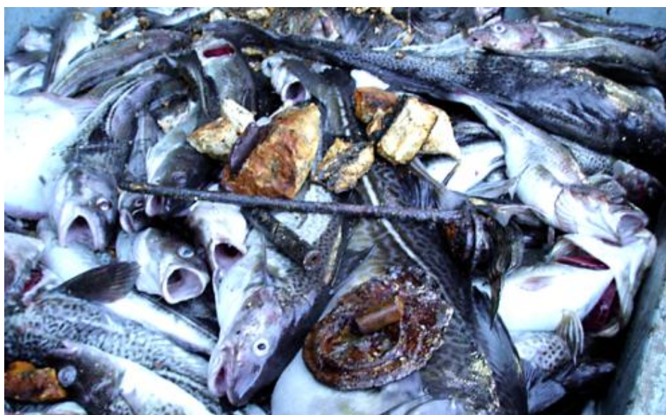
Figure 44: Lumps of solidified sulfur mustard and the metal parts of a Spray Can 37 mine trawled up with a catch that was later discarded (Picture source: Maritime Surveillance Centre South on Bornholm).
