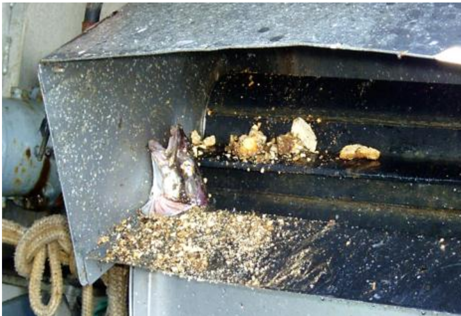
Figure 36: Small lumps of sulfur mustard in the fish conveyor belt on board a fishing vessel. Since it could not be ruled out that some of the particles actually might be explosives, they had to be emergency-relocated ( cf. Chapters 3.2.3.3 & 4.3.1) (Picture source: Maritime Surveillance Centre South on Bornholm).
