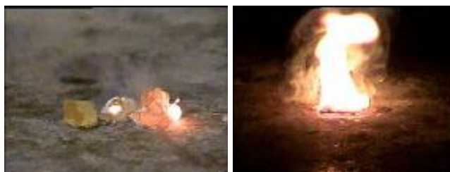
Figure 26: Self-ignition of white phosphorus nuggets (Picture source: Kevin A. Boudreaux, Angelo State University, USA).
