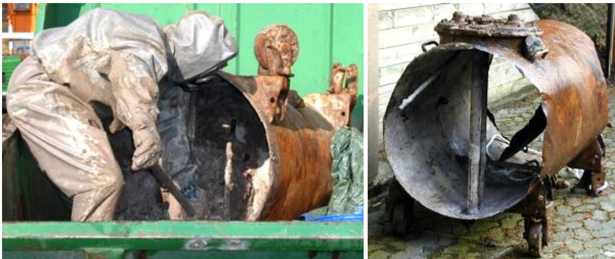
Figure 42: A 900 L container of unknown origin (cf. Figure 27) with 1,057 kg of Clark I-type chemical warfare agent mixture was found in a warehouse in the port of Nexø in 2001 (cf. Annex 7.1 - Table 6).. It was decontaminated and the contents disposed of in a disposal facility (Picture source: Maritime Surveillance Centre South on Bornholm).
