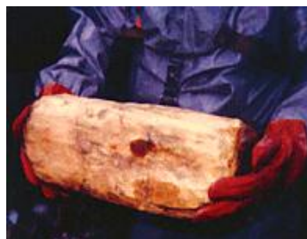
Figure 10: A lump of solidified sulfur mustard from a Spray Can 37 mine, evident by the conserved shape (Picture source: Maritime Surveillance Centre South on Bornholm).
