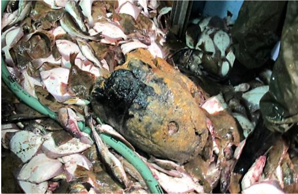
Figure 39: A 45 kg lump of solidified sulfur mustard trawled up with the catch. Since it contained explosives, it was emergency-relocated (Picture source: Maritime Surveillance Centre South on Bornholm).
