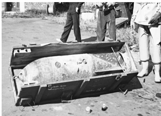
Figure 17: A KC250 aircraft bomb in its wooden storage and transport crate (sides removed and the filling hole of the bomb visible) at Bornholm (Picture source: Bornholm Marinedistrikt).
