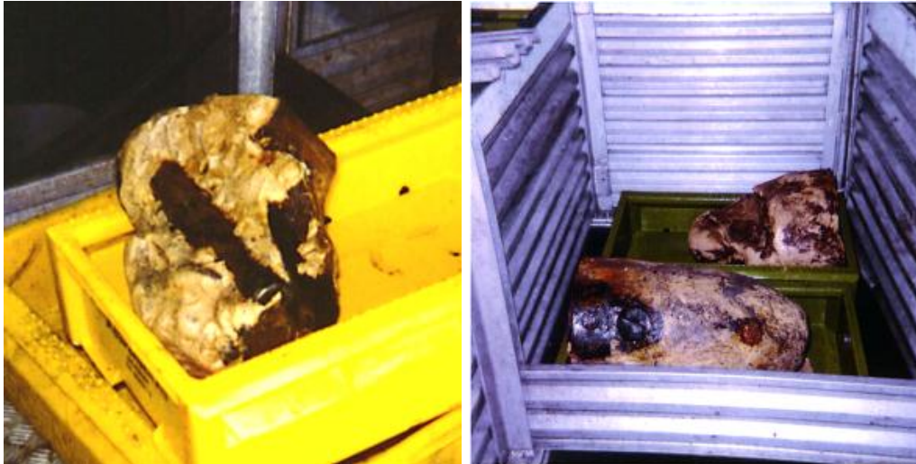
Figure 38: Lumps of solidified sulfur mustard trawled up with a catch. Since they contain explosives (left - bursting charge tube with about 15 kg of explosives visible), they were emergency-relocated ( cf. Chapter 3.2.3.3) (Picture source: Maritime Surveillance Centre South on Bornholm).
