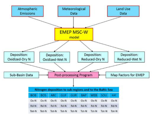
**Figure 9.3.** Computational diagram for calculating oxidized, reduced and total nitrogen deposition to sub-basins of the Baltic Sea and to the entire Baltic Sea Basin using the EMEP MSC-W model.
