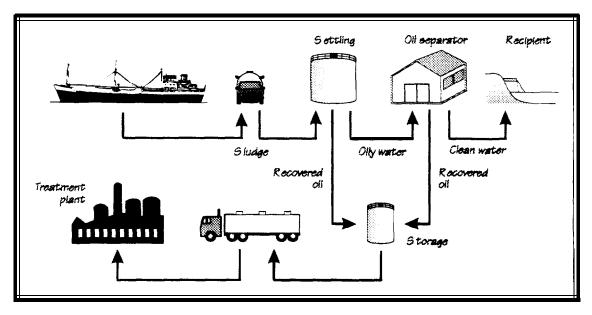
Fig. I. Engineroom wastes from the ship to final processing
