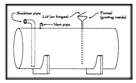
For smaller quantities of oily wastes a tank of a few cubic meters should be provided (fig. 11). The tank should have a fixed funnel at the top. Inside the funnel there should be a grating to prevent oily rags or other debris from entering the tank. The funnel should have a lid and be provided with a pipe
