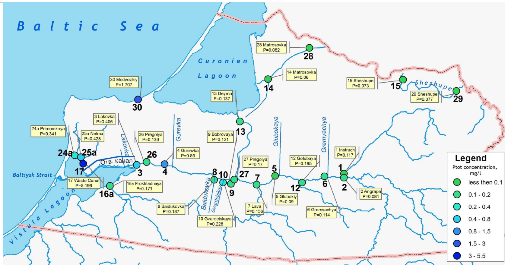
Figure 2.51– Distribution of Total Phosphorus Concentration in Water (mg/l) based on Data Analysis of Samples collected during Summer Low- Water Season
